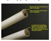
burrs from the ends of each pipe. The inside is not important but the outside should be clean and free of burrs. Set them on end and check that
