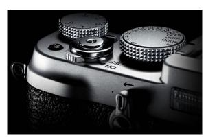
The upper control deck and bottom surface of the camera has been cast from magnesium alloy, (semi-solid metal casting), to create a high-precision body with high rigidity. All dials on the upper control deck are also fabricated from metal.
