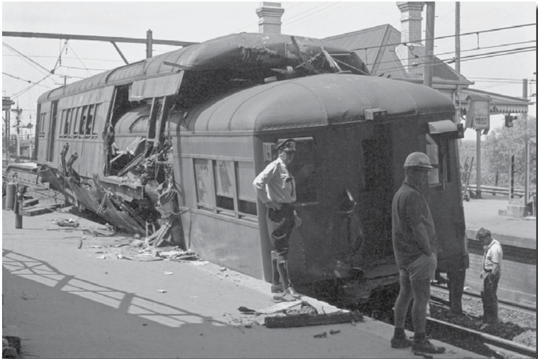
Telescoped carriages at Number One platform Liverpool. On 31 October 1965, a goods train collided with a stationary electric passenger train waiting to depart Liverpool station in Sydney. One person was killed and four people were injured. The cause was the driver of the goods train having fallen asleep Jeff Cutting
