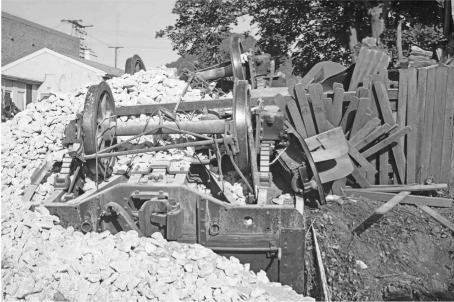
"S" waggon loaded with limestone, one from a whole train, including the locomotive, derailed at Unanderra - 31 December 1962 Jeff Cutting 1963
